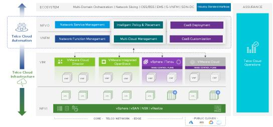
tion to form a cloud-native platform VMware Telco Cloud Platform combines networking and compute with VMware Telco Cloud Auto that runs CNFs and VNFs on any cloud with visibility, orchestration, and operational consistency.
