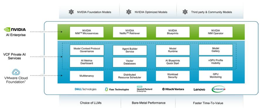
Figure 1: The VMware Private AI Foundation with NVIDIA platform architecture.
