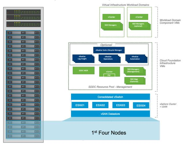
As depicted in Figure 5, the management domain consists of a vSphere cluster, initially with four hosts that is, the first four hosts of the first rack. It hosts management VMs, which can be subdivided into the following areas:
