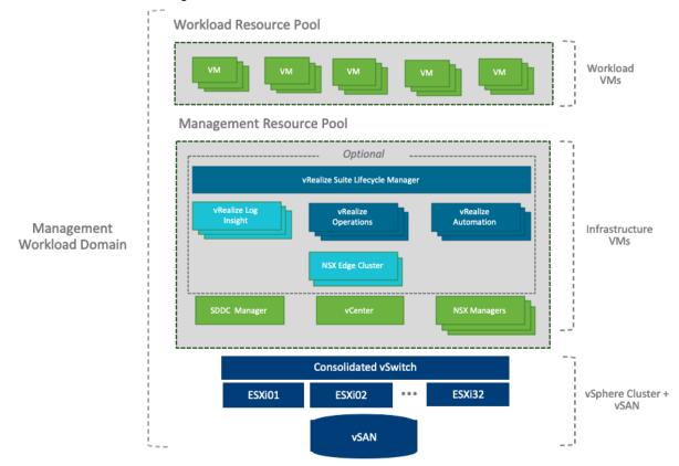
Figure 1. Cloud Foundation Consolidated Architecture
