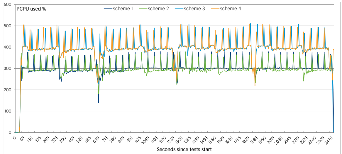
Figure 16. Physical CPU (PCPU) used by the database VMs in the baseline experiments in Figure 12
