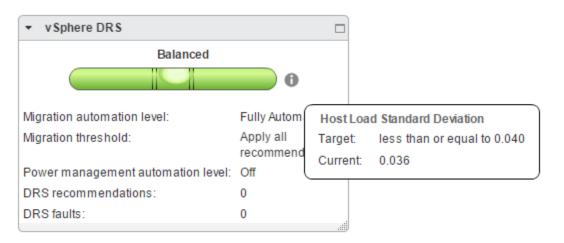
Figure 45 - Cluster Balance Host Load Standard Deviation after DRS balances cluster
