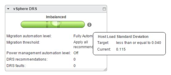
Figure 43 - Cluster balance Host Load Standard Deviation when DRS Threshold is set to 5
