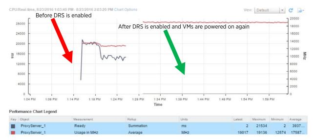
Figure 19 - CPU Ready Time before and after DRS is enabled
