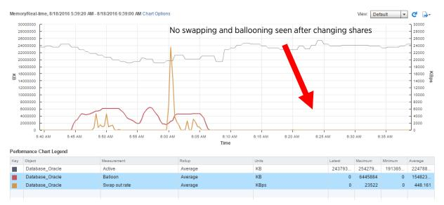
Figure 39 - Chart showing VM memory pressure reduced for high priority VM
