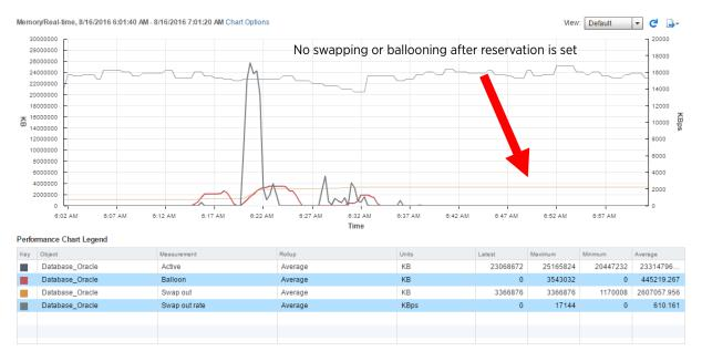
Figure 33 - VM Memory Graph showing no ballooning and swapping after reservation is set
