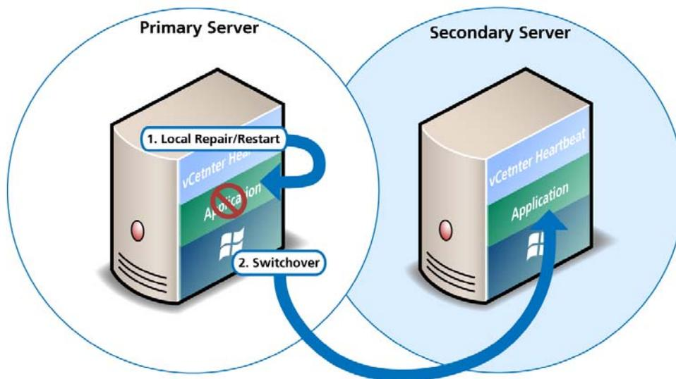
A switchover gracefully closes any protected applications that are running on the active server and restarts all of them on the passive server, including the application or service that caused the failure as illustrated in [Figure 1-2](#).
