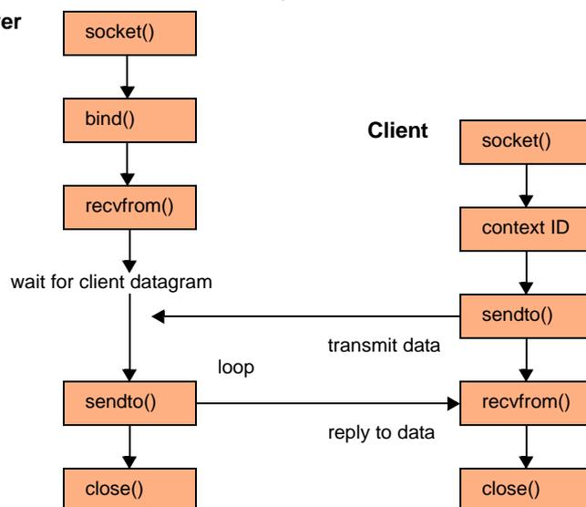
In UDP sockets, the server waits for the client to transmit, and accepts datagrams. In VMCI sockets, the server and client communicate similarly with datagrams.
