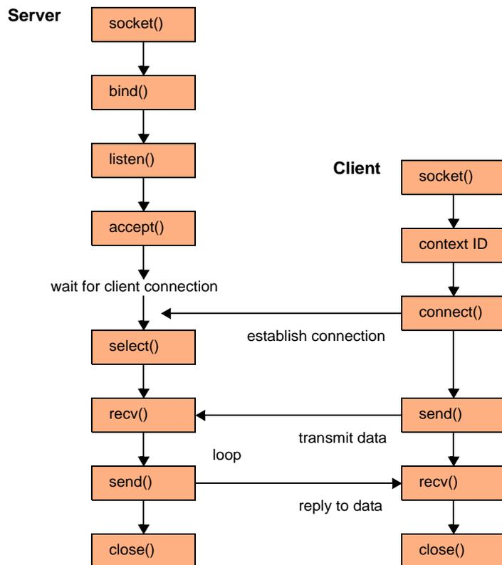
With VMCI sockets and TCP sockets, the server waits for the client to establish a connection. After connecting, the server and client communicate through the attached socket. In VMCI sockets, a virtual socket can have only two endpoints, and the server cannot initiate a connection to the client. In TCP sockets, more than two endpoints are possible, though rare, and the server can initiate connections. Otherwise, the protocols are identical.
