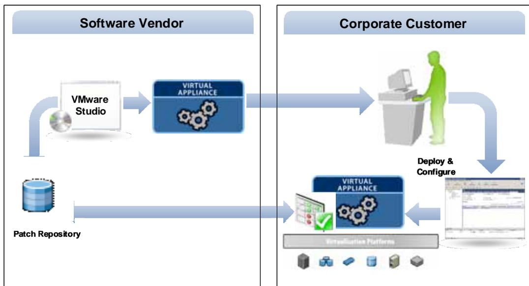
VMware Studio provides both a Web interface and a command-line interface to build virtual appliances. The Web interface offers ease of use and online help. The command line interface can integrate with existing source control or configuration management systems for fully automated builds of virtual appliances.
