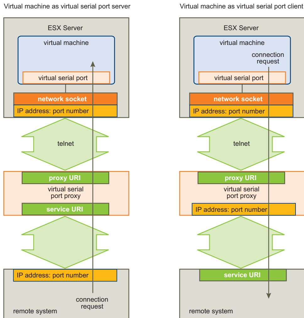
Figure 1-2. Virtual Serial Port Connections to a Remote System Through a Proxy
