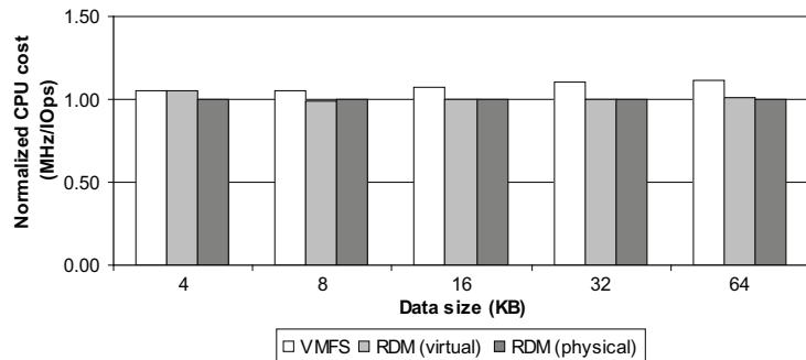
**Figure 10.** Normalized CPU cost for sequential read (lower is better)
