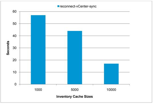
Figure 22. Sync Time for Inventory Cache Sizes Set to 1000, 5000 and 10,000 with 5000 VMs
