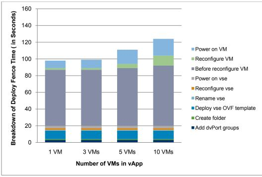
Figure 18. Deploy a Single vApp with Fence Mode: Operation Breakdown
