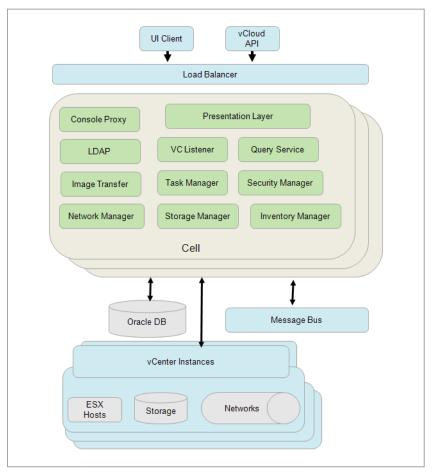
Figure 2 shows the internal architecture of vCloud Director. Performance results for LDAP, Image Transfer (OVF File Upload), and VC Listener are included in this paper.
