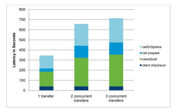
Figure 8. OVF Uploads with 1, 2, and 3 OVF Packages Transferring at the Same Time
