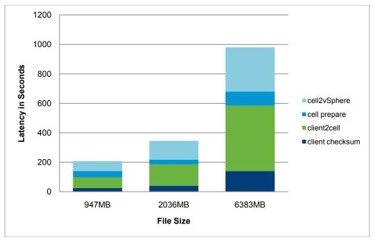
Figure 7. OVF File Upload Latency Breakdown for Different File Sizes
