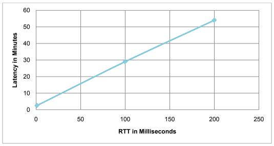
Figure 4. LDAP Sync Latency for Round-Trip Time (RTT) with 10,000 LDAP Users = 1ms, 100ms, and 200ms
