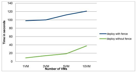
Figure 17. Deploy a Single vApp with and without Fence Mode
