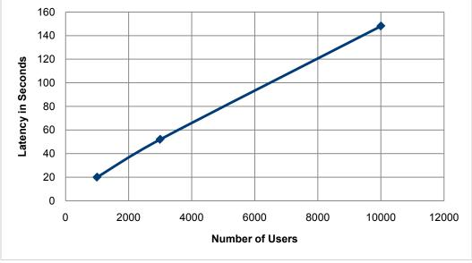
Figure 3. LDAP Sync Latency in Seconds for 1000, 3000, and 10,000 LDAP Users
