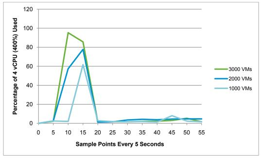
Figure 23. vCenter CPU Usage for Reconnect-vCenter-Sync with 1000, 2000 and 3000 VMs
