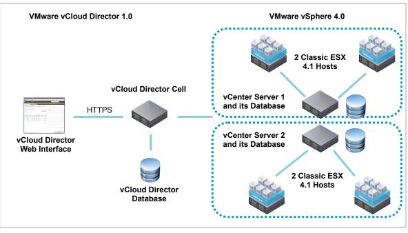
Figure 11. Testbed Setup for Inter-vCenter Clone Experiments
