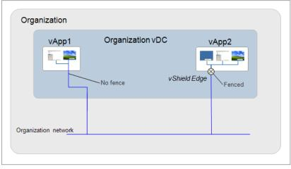
Figure 16. vApps Deployed with and without Fence Mode
